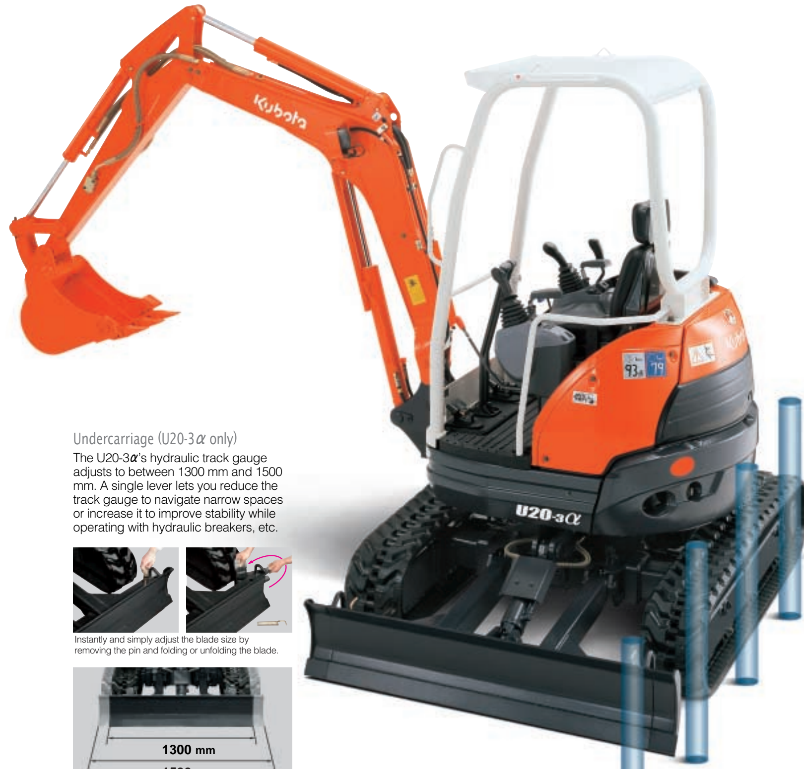
Increase the track gauge for greater stability, or reduce it to navigate narrow spaces.
