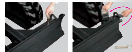
Instantly and simply adjust the blade size by removing the pin and folding or unfolding the blade.
