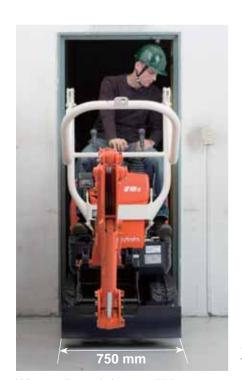
When adjusted down to 750 mm, the U10-3 can easily fit through most doorways, permitting access inside of buildings.
