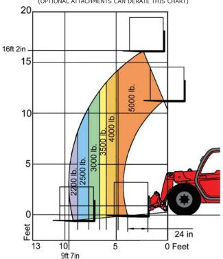
Capacities shown in pounds/feet are the maximum recommended load limits at the indicated extensions of the boom. Capacity ratings are based on a 48" homogeneous cube and are in accordance with ANSI/ASME B56.6 stability standards. Capacity reductions must be made for extended load centers and when used with various other attachments, contact MANITOU NORTH AMERICA, INC.
