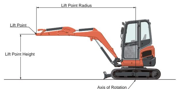
\* Working ranges are with Kubota standard bucket, without quick coupler.
