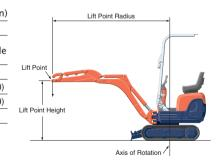
Please note: \* The lifting capacities are based on ISO 10567 and do not exceed 75% of the static tilt load of the machine or 87% of the hydraulic lifting capacity of the machine.
